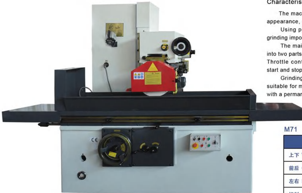
Surface grinding machine with horizontal spindle and rectangular table
